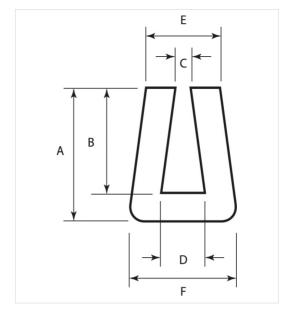
Made from self-extinguishing PVC, this material has excellent flexibility which makes application quick and easy. A halogen-free type is now also available for use in critical areas.
